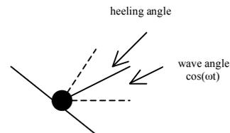
Thus, the roll angle is created by both the wave face and by the boat's roll time. Denny (2008)<sup>8</sup> shows, with some simplifying assumptions, that the roll angle from both sine waves and heeling is
